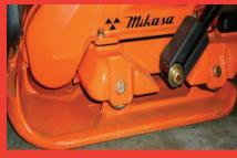
**Baseplate Design -** open for easy removal of rock build up and special contour for asphalt applications.
