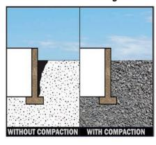
Figure 3 — These illustrations show the results of improper compaction and how proper compaction can ensure a longer structural life, eliminating future foundation problems.
