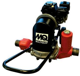
3" Suction/Discharge • 90 GPM Flow • 25' Head 1-5/8" Solids • Honda GX120, 3.5 HP
